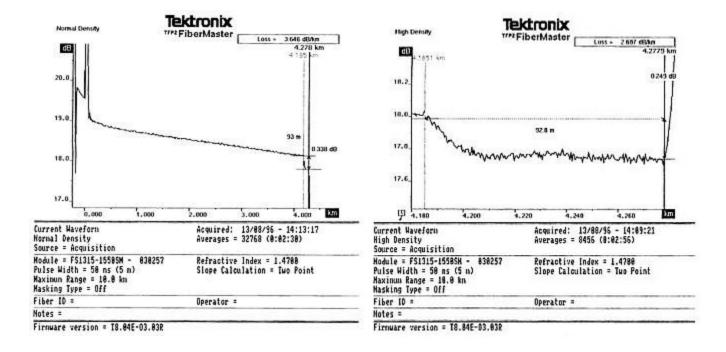
Fig 11.2: Trace of the fault & Cold Clamp loss.
