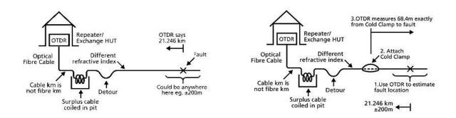
Fig 11.1: A typical requirement for the use of a Cold Clamp.
